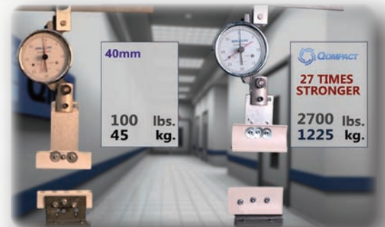
Pull-Apart Strength Test with 152mm (6in.) Sample. Qcompact Pull Apart at 8050 kg/m 40mm Pull Apart at 296 kg/m
