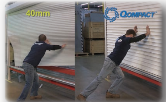
Qcompact's end retention prohibits the curtain from being pushed out of the rails. Without end retention, the 40mm foam-filled curtain was easily compromised.
