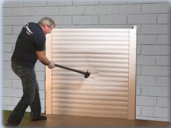
In impact testing, Qcompact withstood 82 punches, 5 kicks, and 80 hits with a sledge hammer. The foam-filled shutter was destroyed in seconds.
